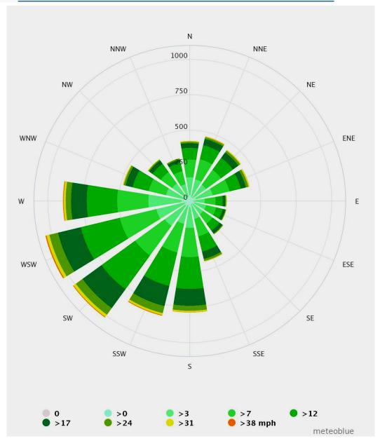
The wind rose for Bristol shows how many hours per year the wind blows from the indicated direction. Example SW: Wind is blowing from South-West (SW) to North-East (NE).about
